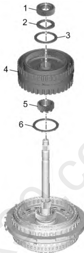
Fig. 17: Exploded View Of O/D And Reaction Carrier Components Courtesy of GENERAL MOTORS COMPANY
